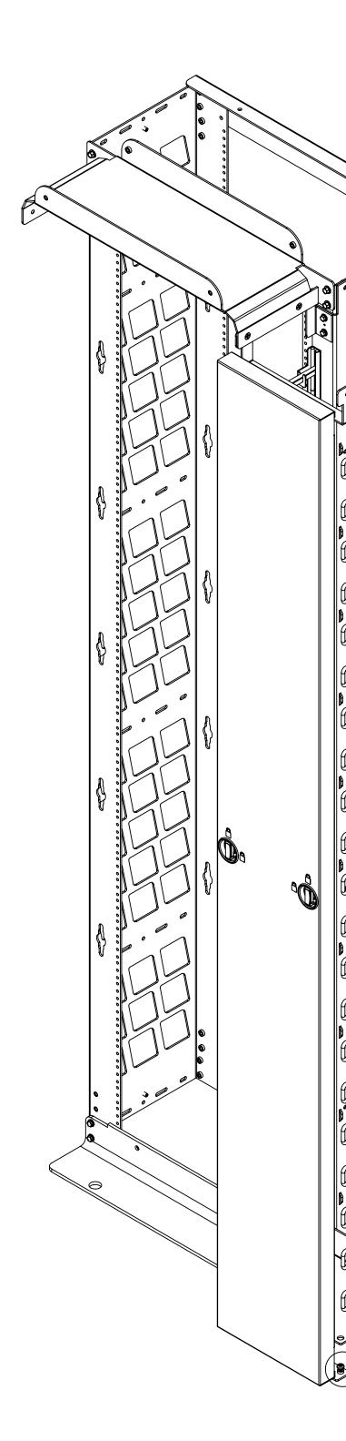
STEP 2: TURN STEP 1: INSERT WIRE FINGERS WIRE FINGERS SO THEY ARE IN AT AN ALIGNED ANGLE VERTICALLY ABOVE HOOKS STEP 2: ALIGN WIRE FINGERS STEP 3: DROP FINGERS DOWN WITH HOOKS IN INTO SLOTS BRACKET
