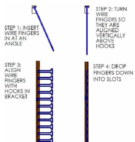
**SEE SHEET 2 FOR ALTERNATE** MOUNTING FOR FINGERS ON INSIDE
