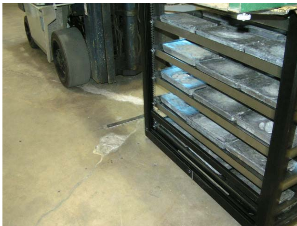
Photo 2: Steel Floor Hazard
