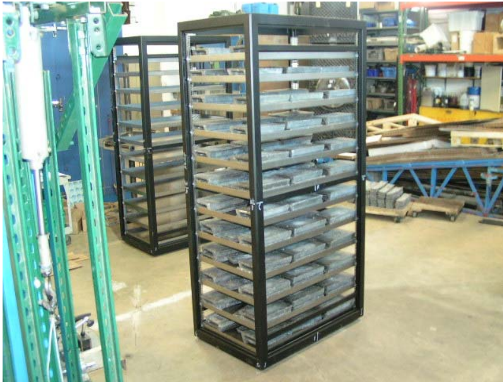
Photo 5: Static Loading with 8484 Lbs. Total Load
