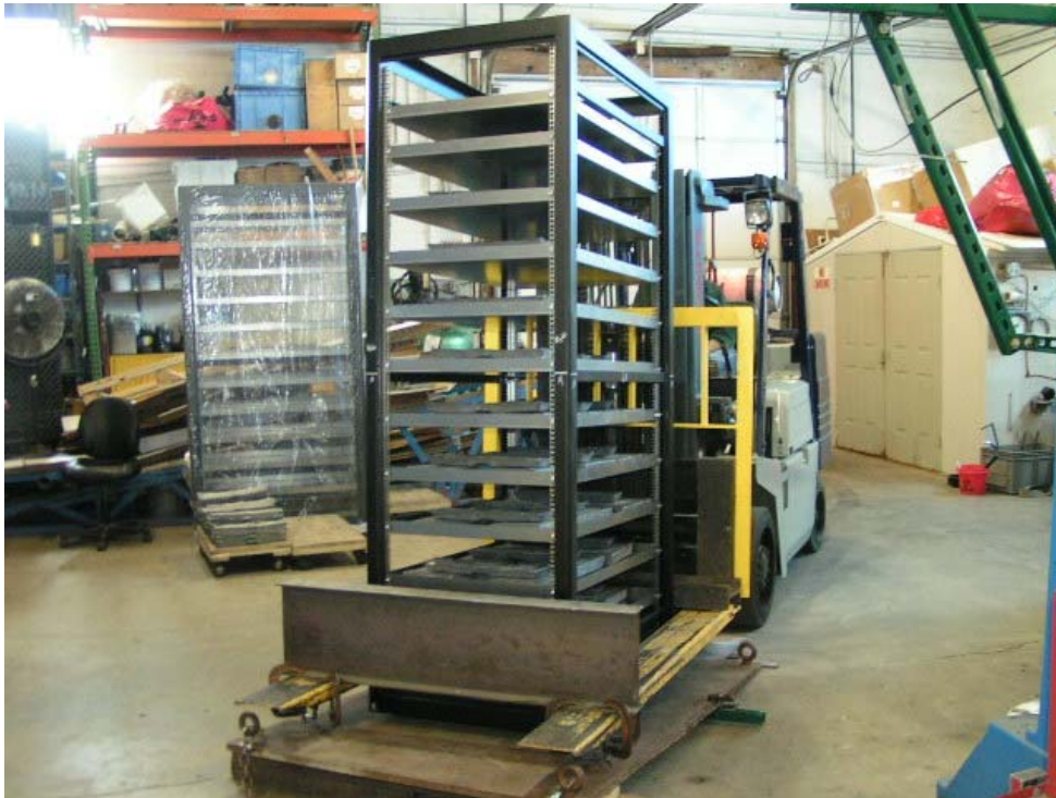
Photo 3: Frame Loaded with 4464 Lbs. on 5° Incline
