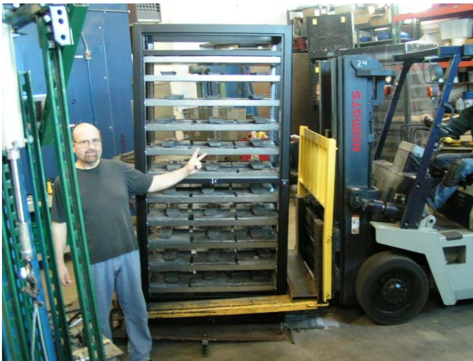
Photo 4: Frame Loaded with 5304 Lbs. on 5° Incline, 2nd Test
