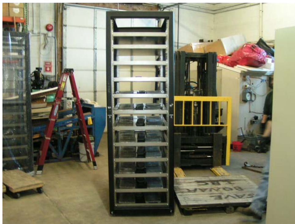
Photo 1: 4464 lb. Load on Frame for Dynamic Testing
