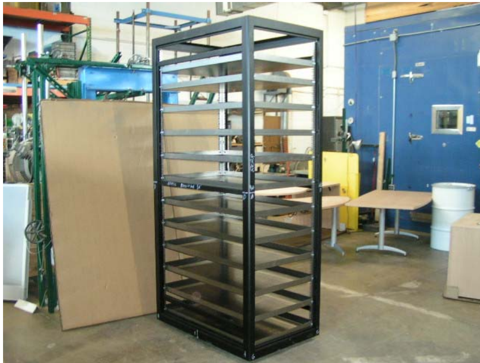
Photo 12: Condition of Frame after Static Loading to 8484 Lbs.
