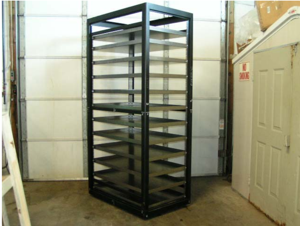
Photo 11: Condition of Frame after Dynamic Loading to 4464 and 5304 Lbs.
