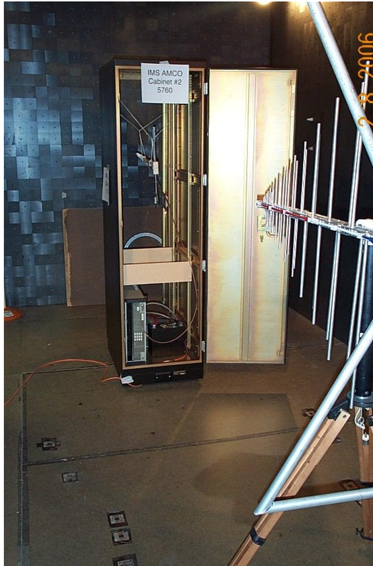
Figure 4. Photograph of Plane wave Shielding Test (30 to 1000 MHz)
