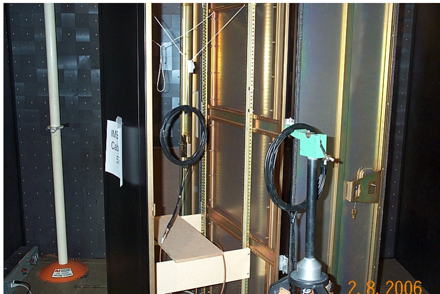
Figure 2. Photographs of H-field Shielding Test (0.01 to 10 MHz)
