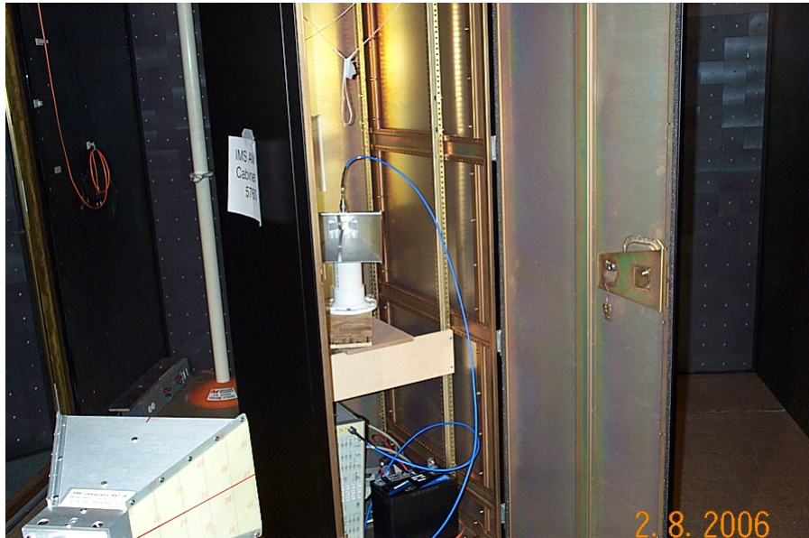
Figure 5. Photograph of Plane wave Shielding Test (1 to 18 GHz)
