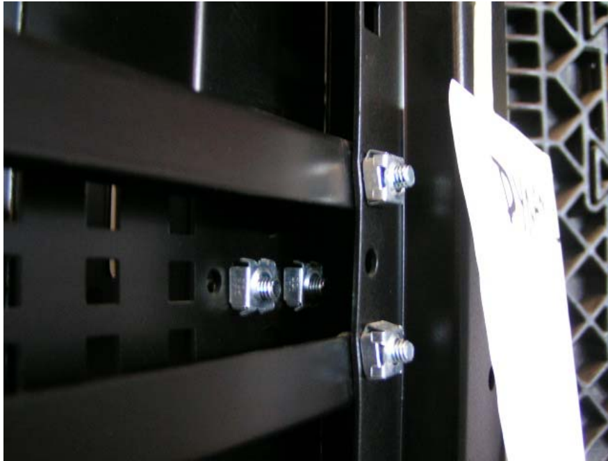
Photo 9: Distortion of vertical corner frames during 3200 lb. Dynamic Load Test.
