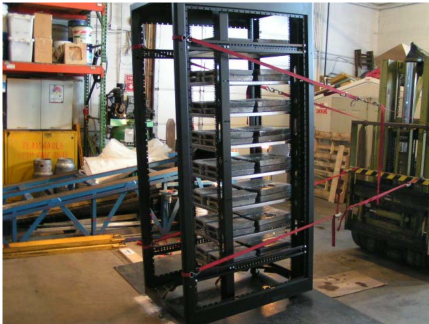
Photo 4: Cabinet Loaded with 3200 Lbs. on 5° Incline
