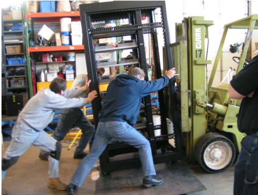
Photo 3: Cabinet Loaded with 2400 Lbs. on 5° Incline
