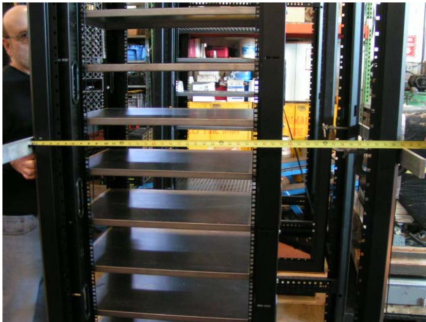
Photo 10: Measuring technique between vertical corner frames.
