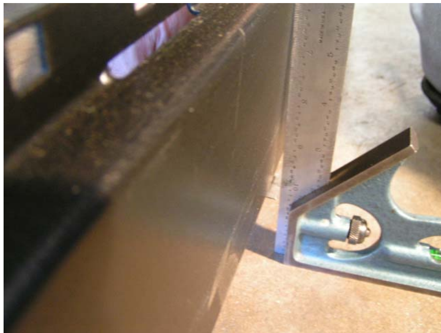
Photo 6: Measuring Technique to Determine Distortion of Vertical Alignment
