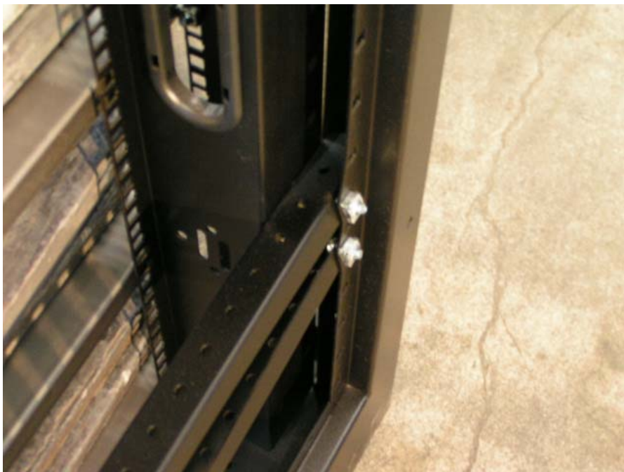
Photo 14: Distortion of the vertical corner frame and lower horizontal side rail.
