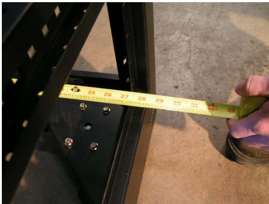
Photo 8: Measuring Technique Between the Lower Frame Rails
