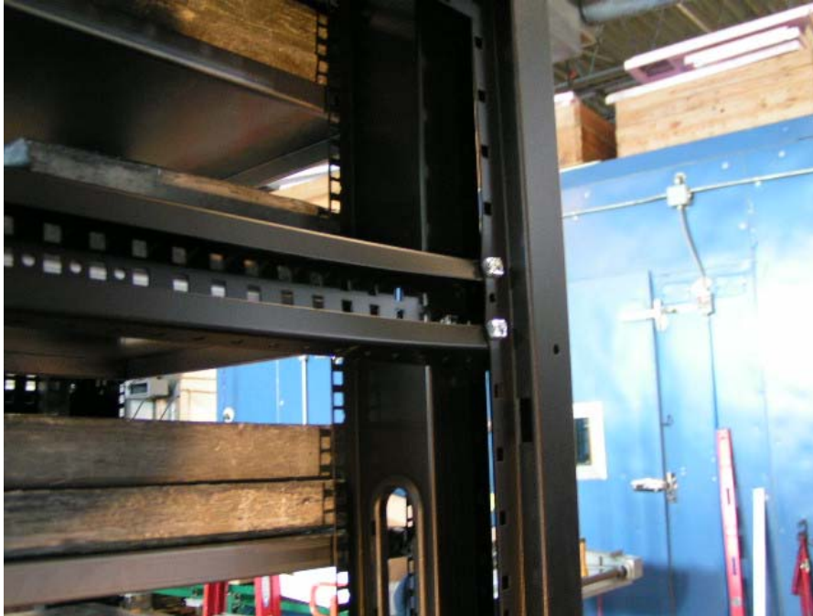
Photo 13: Distortion of the vertical corner frame and upper horizontal side rail.
