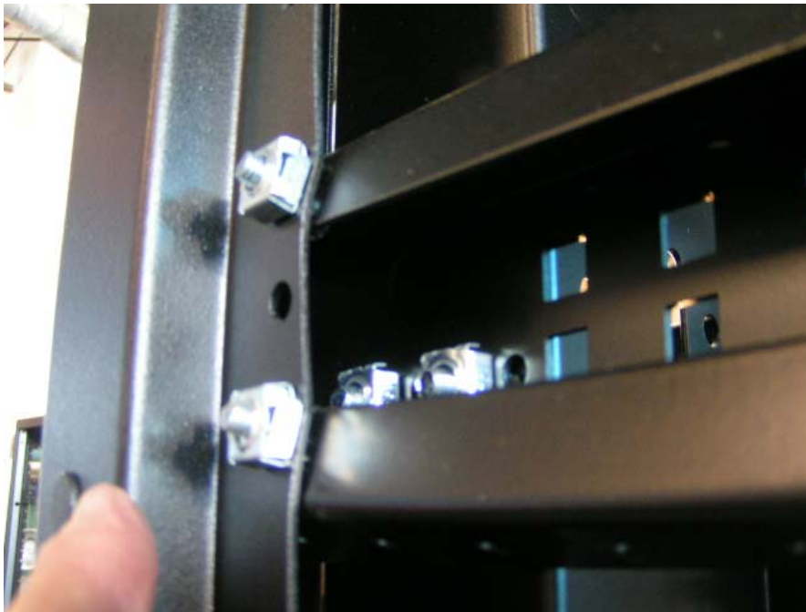
Photo 12: Distortion of the vertical corner frame and horizontal side rails.
