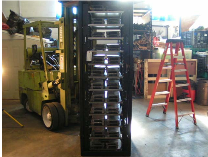
Photo 5: Static Loading with 4800 Lbs. (400 lbs./Shelf)
